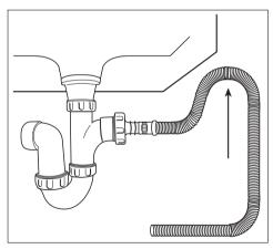
**Important!** Before connecting up the machine to new pipework or to pipework that has not been used for some time, run off a reasonable amount of water to flush out any debris that may have collected in the pipes.
